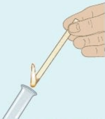
Figure 4.14 A flaming splint will be extinguished in the presence of carbon dioxide.
