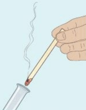
Figure 4.13 A glowing splint will reignite in the presence of oxygen.
