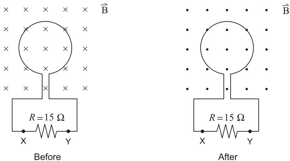
What are the magnitude and direction of the current through the  $15 \Omega$  resistor?
